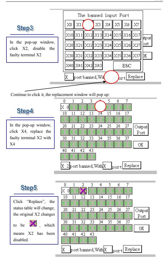
As in the above graphs, we need only 5 minutes replace I/O terminals. This method avoids us to modify the program, change PLC etc.
